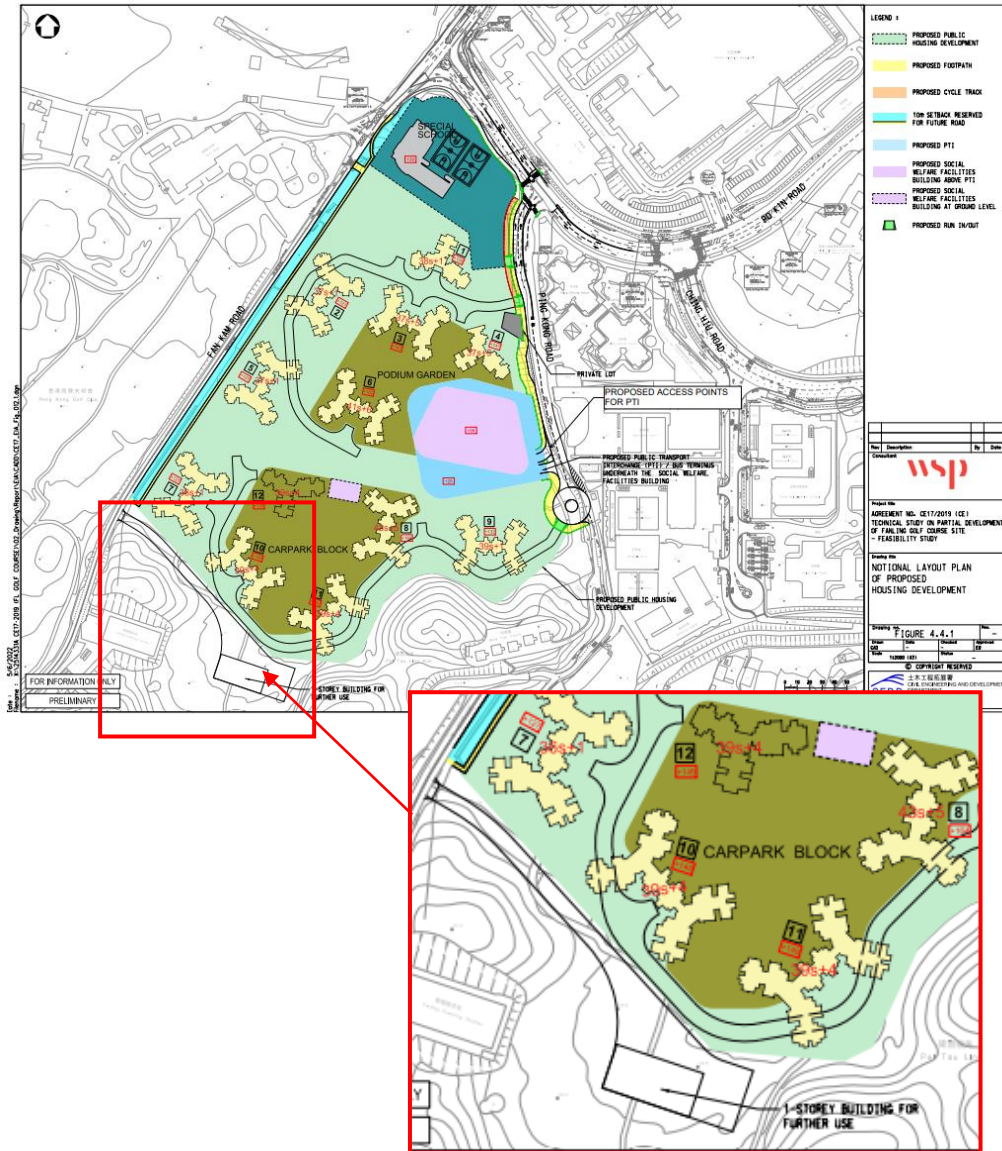
Figure 1 The notional layout plan (Appendix 11.4) reveals that a 1-storey building and an associated vehicular access (marked in red) are proposed in Sub-Area 2
